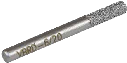
DOME END ROUTER Tool length 60mm, with a 6mm shank, 6mm diameter & a 19mm coating of diamond. • High grade diamond. • 44/60 grit. • Nickel coated blank.
