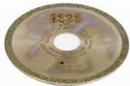
DIAMOND WHEEL • High grade diamond. • 44/60 grit. • 5mm wrapover. • Nickel coated blank. • Hardened, ground and balanced blank
