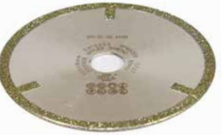
DIAMOND WHEEL (SIDE SPOKED) • High grade diamond. • 44/60 grit. • 5mm wrapover. • Nickel coated blank. • Hardened, ground and balanced blank.
